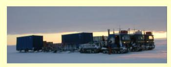
SWEDARP (Swedish Antarctic Research Programme) has three TL4 vehicles, the forerunner to the new TL6. SWEDARP use the TL4 vehicles, they also use a lot of sledges and 20-foot accommodation modules in their logistic system. Sledges and modules for different uses are made by Berco
